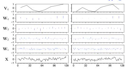
• Haar DWT of FD(0.45) series **X** (left-hand column) and wavelet-domain bootstrap thereof (right-hand)
