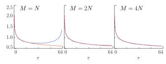
• plot shows true ACVS  $\{s_{X,\tau}\}$  (thick curves) for FD(0.4) process and wavelet-based approximate ACVSs  $\{s_{\widetilde{Y},\tau}\}$  (thin curves) based on an LA(8) DWT in which an N = 64 series is extracted from M = N, M = 2N and M = 4N series
