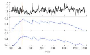
• Nile River minima (top plot) along with curves (constructed per Equation (382)) for scales  $\tau_1 \& \tau_2$  (middle & bottom) to identify change point via time of maximum deviation (vertical lines denote year 715)
