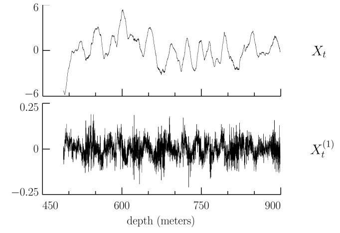
• selected 'stationary' portion of vertical shear measurements  $\{X_t\}$  (top plot) and their first backward differences  $\{X_t^{(1)}\}$
