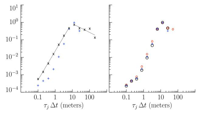
• unbiased MODWT wavelet variance estimates using the following wavelet filters: Haar (**x**'s in left-hand plot, through which two regression lines have been fit); D(4) (small circles, righthand plot); D(6) (pluses, both plots); and LA(8) (big circles, right-hand plot).
