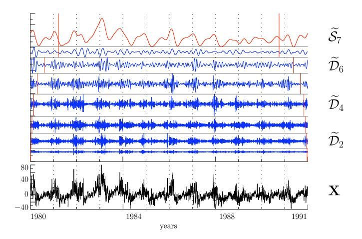
• level  $J_0 = 7 \text{ LA}(8)$  MODWT multiresolution analysis
