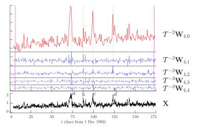
• level j = 4 LA(8) DWPT coefficients  $\mathbf{W}_{4,n}$ ,  $n = 0, \dots, 4$ , after time alignments (derived from study of phase functions)
