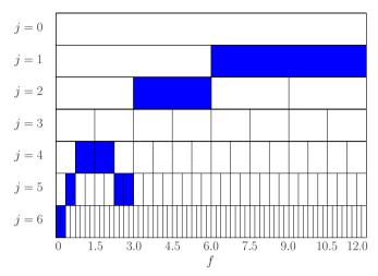
• best basis transform using LA(8) filter and  $-W_{j,n,t}^2 \log(W_{j,n,t}^2)$  cost function
