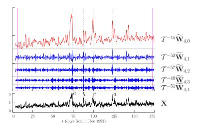
• level j = 4 LA(8) MODWPT coefficients  $\mathbf{W}_{4,n}$ ,  $n = 0, \dots, 4$ , after time alignments
