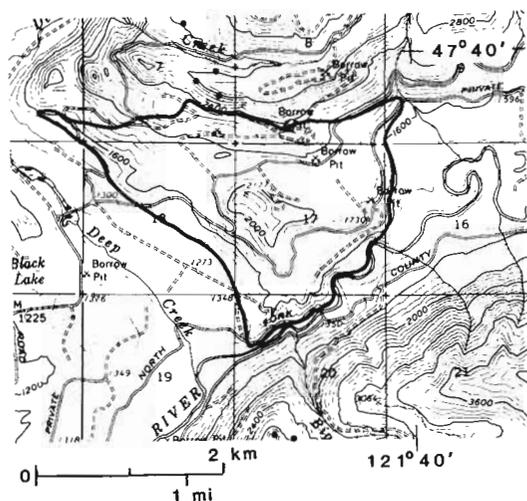
Fig. 3. North Fork Snoqualmie embankment (outlined). Post-depositional erosion is evident both in the transverse incision by the North Fork Snoqualmie River (N 1/2 section 20) and by modification of the ice-proximal face by recessional meltwater flowing south down the valley of Deep Creek (Sections 18-19). Topography from USGS Mount Si 15' quadrangle. Ice-maximum limit shown by black dots; altitude in feet.
