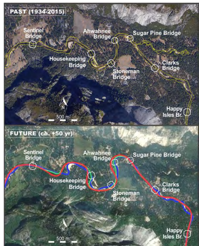
FIGURE 6 Channel migration patterns of the Merced River. Past changes shown by superimposing the 1934 channel position (top panel, yellow outline) on the 2015 Google Earth airphoto. Future changes from the channel centerline in 2016 (bottom panel, blue line) are modelled, with four main areas of existing revetments included (green line) and omitted (red line). The dominant mode of future change is downvalley meander migration where revetments have been removed (i.e., where the red and green lines diverge), with one location of anticipated avulsion between Housekeeping and Sentinel bridges [Color figure can be viewed at wileyonlinelibrary.com ]
