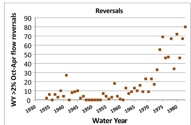
**FIGURE 9** Water-year (WY) values of the three hydrologic metrics for Arroyo Simi (USGS gage 11105850). Only the pattern of flow reversals is consistent with mid-century advent of watershed urbanization (Hawley & Bledsoe, 2011); both  $T_{Qmean}$  and Richards-Baker Index (RBI), if naively interpreted, would imply an early record increase in flashiness followed by a marked decline. Missing or zero values, particularly in the early 1950s, are years of no recorded flow at all
