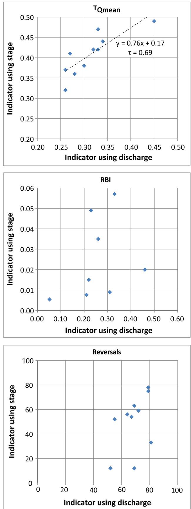
**FIGURE 11** The three hydrologic metrics recommended for use, comparing the decadal-averaged values for each site calculated using the discharge record (x-axis) and the stage record (y-axis). Only  $T_{Qmean}$  shows a useful relationship with the data as they are presently archived. RBI = Richards-Baker Index
