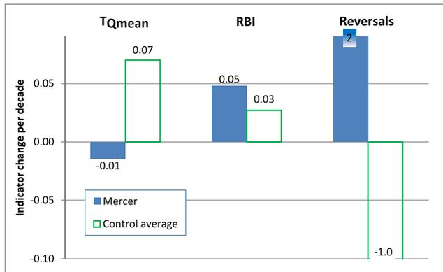
**FIGURE 8** Average rate of change in hydrologic metrics for Mercer Creek over the full period of record (water year 1956–2016, with control-site averages from the last decade provided for reference). All Mercer Creek changes are consistent with increasing urbanization, supporting an inference of long-term increase in flashiness corresponding to the multidecadal period of urbanization in the watershed. RBI = Richards-Baker Index
