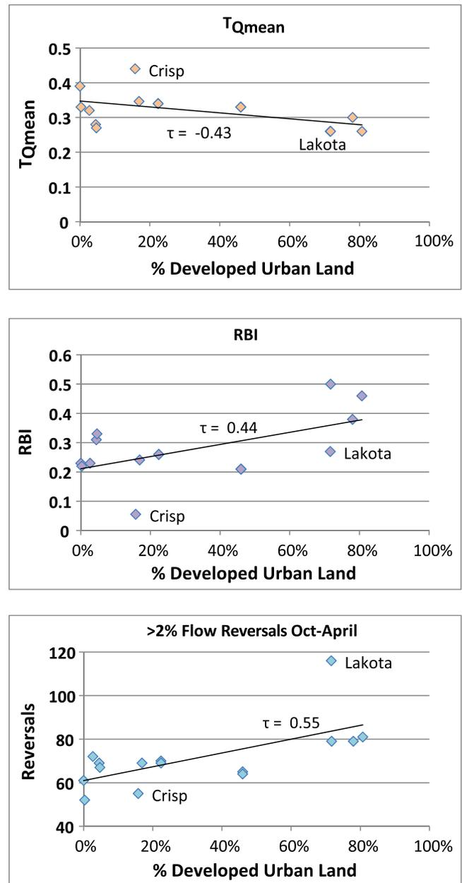
**FIGURE 2** All sites with analysed hydrologic data, with the specified metric plotted against the 2011 watershed urban land cover (all *p* values <0.05). Each point is a single site, calculated for each individual water year independently, with all annual values then averaged over the full period of record. The two labelled sites (Crisp and Lakota) display somewhat anomalous relationships relative to the trends established by the others. RBI = Richards-Baker Index
