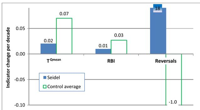
**FIGURE 6** Decadal rate of change in hydrologic metric values for Seidel Creek, extrapolated from the period 2009–2015. Trends in this watershed imply *less* hydrologic changes than those expressed for the control sites using T<sub>Qmean</sub> or Richards-Baker Index (RBI); however, the trend for reversals is dramatically more rapid (i.e., more urban) than for those same control sites
