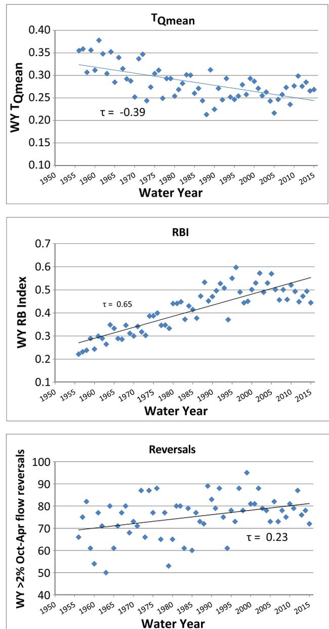
**FIGURE 7** Water-year (WY) values of the three hydrologic metrics for Mercer Creek (USGS gage 12120000), the longest record in the data set (all  $p$  values <0.01). RBI = Richards-Baker Index
