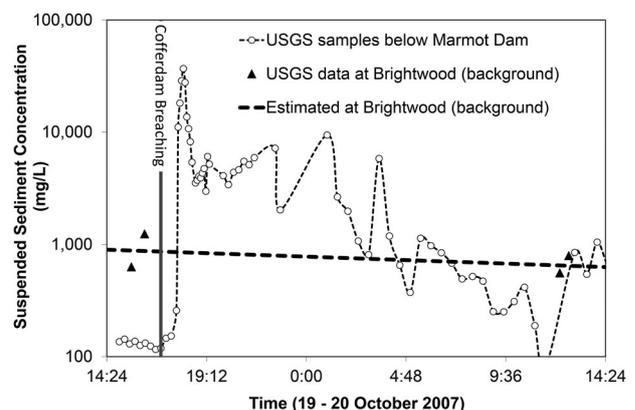
**Figure 7.** Measured suspended sediment concentration in Sandy River downstream of Marmot Dam during cofferdam breaching after Marmot Dam removal. Suspended sediment concentrations were derived from data provided by Major *et al.* (2012) and Cui *et al.* (2014).
