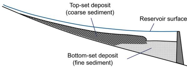
**Figure 1.** Sketch of a typical reservoir deposit, showing the coarse top-set deposit and fine bottom-set deposit.
