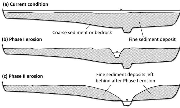
**Figure 8.** Sketches illustrating Phase I and Phase II erosion following Matilija Dam removal. (a) Current condition; (b) Phase I erosion when fine sediment is directly accessible to the flow, presenting a virtually unlimited supply of sediment with transport limited only by the capacity and rate of discharge; and (c) Phase II erosion when fine sediment is no longer directly accessible to the flow.
