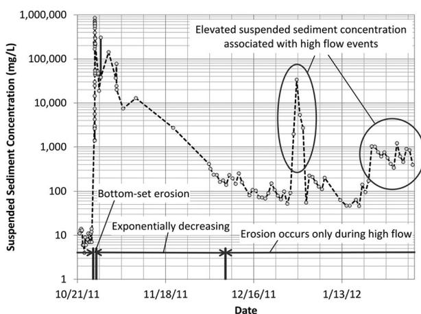
**Figure 6.** Measured suspended sediment concentration in White Salmon River at approximately 2.3 km downstream of Condit Dam during Condit Dam removal, showing different phases of sediment erosion. Suspended sediment data were provided by Wilcox *et al.* (2014).
