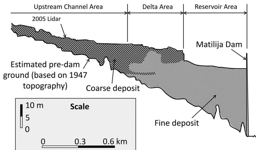
**Figure 5.** Interpreted longitudinal profile of sediment deposits within Matilija Dam impoundment, modified from Stillwater Sciences (2014).
