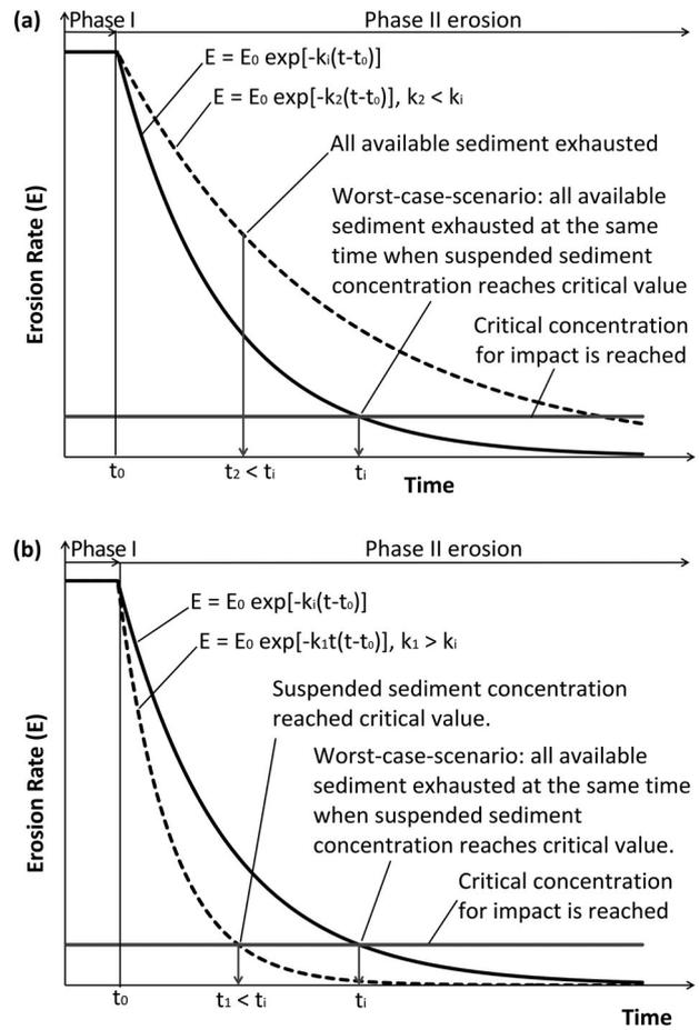
**Figure 10.** Illustration of the concept of maximum potential duration for Phase II erosion. (a) A slower decrease in erosion rate would result in a quicker exhaustion of sediment source; and (b). a faster decrease in erosion rate would result in a quicker realization of critical suspended concentration for impact.
