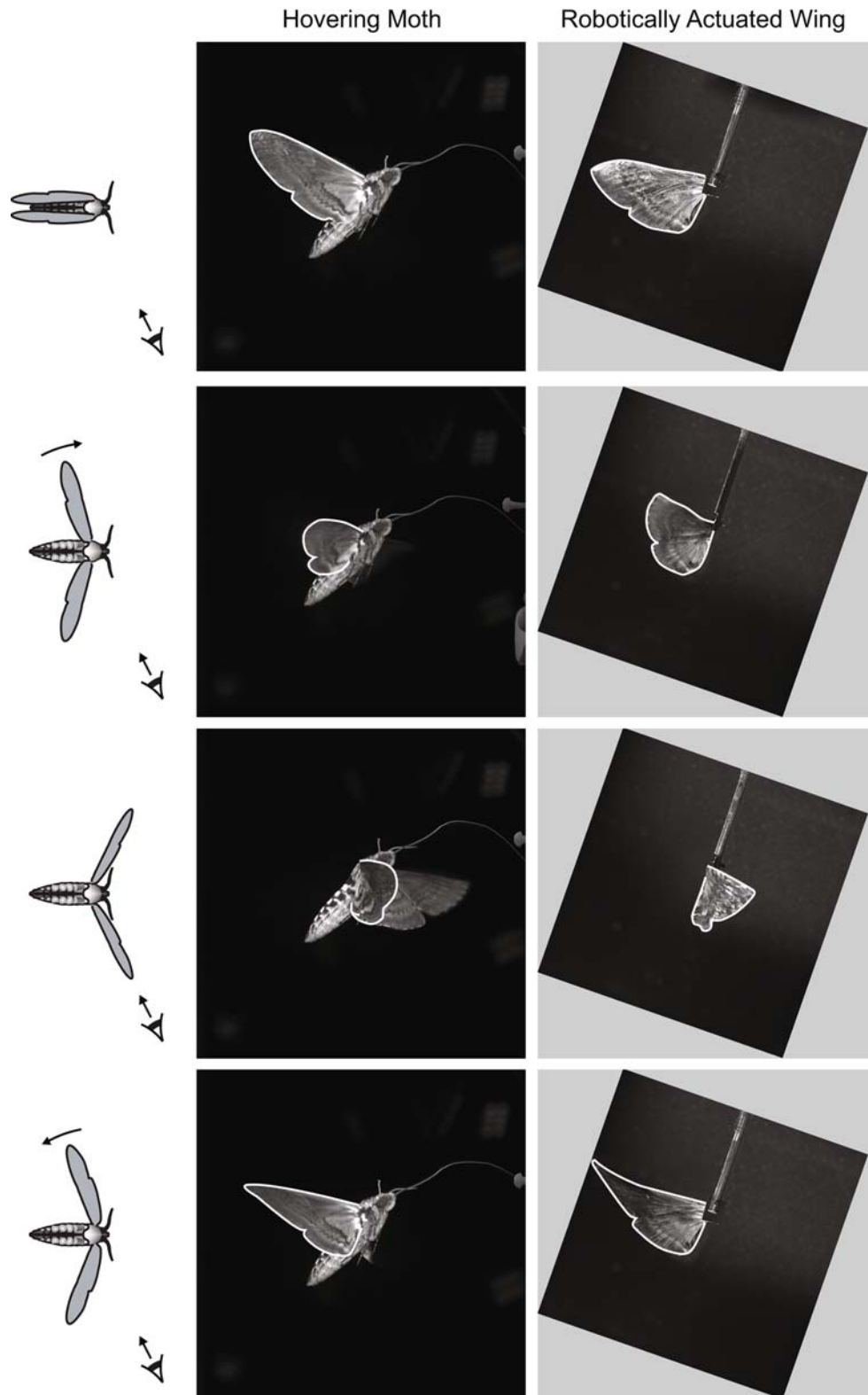
Fig. 4 A freshly extracted wing robotically flapped along a single axis of rotation approximates natural wing motion during hovering flight, illustrated in synchronized phases of a wing stroke at quarterly intervals. The collective tilt of the robotically actuated wing images is the result of a coordinate rotation to match the robotic wing stroke plane with the average stroke plane in hovering flight. The wings have been outlined to highlight their overall similarities in shape. The moth planform diagrams in the left column provide positional reference of the wing stroke phase relative to the viewpoint
