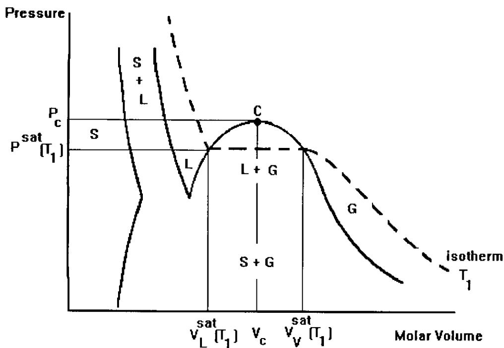
Pressure-Temperature and Pressure-Volume Projections for a Typical Pure Substance
