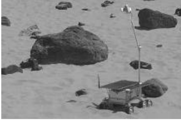
Figure 1: Rocky 7 generating a range map in the JPL Mars Yard using its mast cameras.
