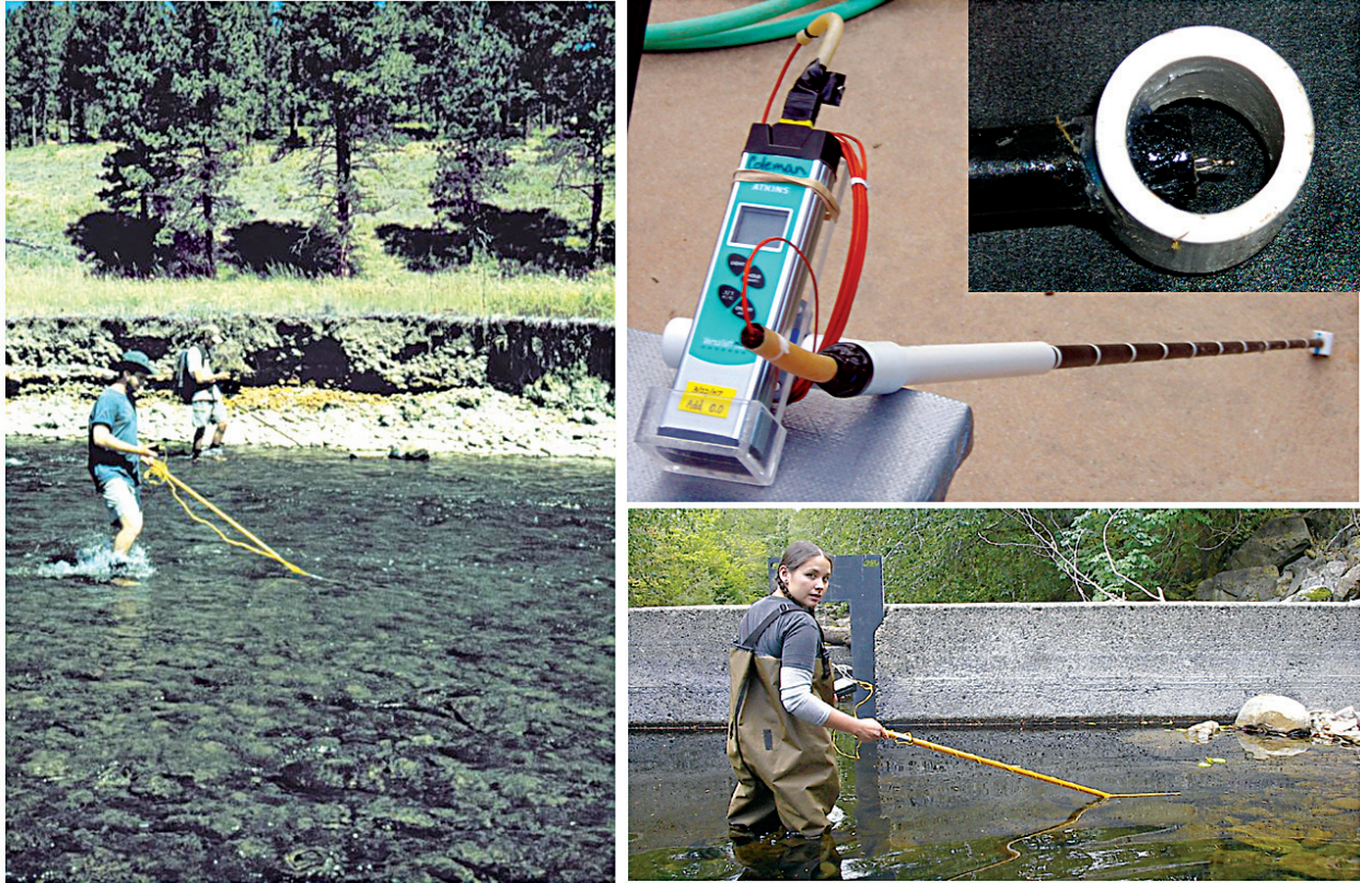
Figure 6.4.1.1. Rapid temperature assessment in wadeable streams with fast-response thermocouple probes. Locations of cold-water areas can be identified by walking through or along the stream and sweeping the extendable probe along the stream bottom. The near instantaneous response of the thermocouple and digital readout of the instrument (Atkins, Inc., Models 35200 and 39658) are essential for identifying thermal anomalies with the pole-mounted probe. Photographs taken by J. Ebersole in 1997, Mark Coleman in 2009 (Coleman Ecological, Inc., personal commun.), and Nancy Raskauskas in 2004 (Oregon State University). http://www.techinstrument.com/acatalog/Digital_Thermometers_Thermocouple.html
