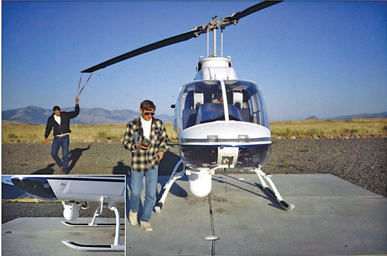
Figure 6.3.3.1. Helicopter and gimbal mount (inset) for airborne TIR remote sensing of stream temperature. The thermal imager (8–14 \mu\text{m} wavelength) and paired daylight video camera (lower left inset) are controlled from inside the aircraft and are georeferenced with a global positioning system (GPS) (for more detail see Torgersen and others, 2001228 and Handcock and others, in press). Photographs taken in 1995 by C. Torgersen. 105
