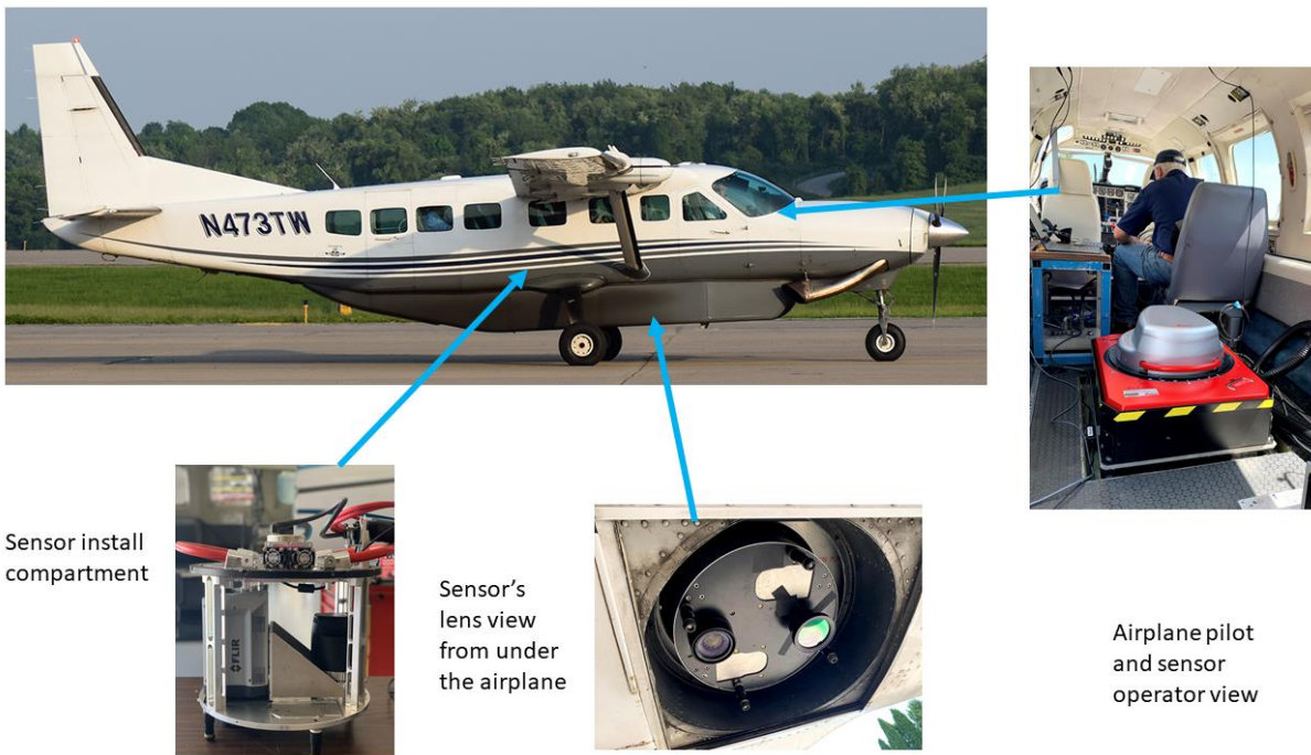
Figure 2: Installation setup of FLIR x8501SC SLS in the fixed-wing aircraft used for Salmon Streams project.
