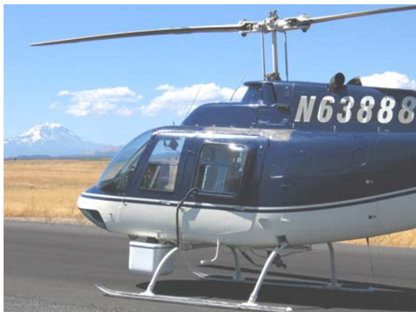
Figure 2 – Bell Jet Ranger equipped with a thermal infrared radiometer and high resolution digital camera. The sensors are contained in a composite fiber enclosure attached to the underside of the helicopter and flown longitudinally along the stream channel.
