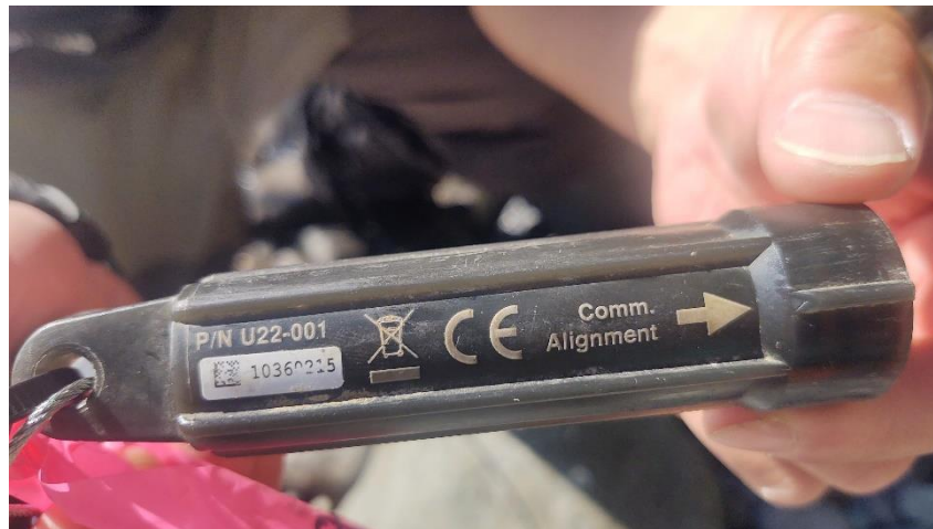
Figure 3: Water temperature data logger that was used for the project. Brand and model: HOBOTemp Pro V2 ONSET U22-0011.
