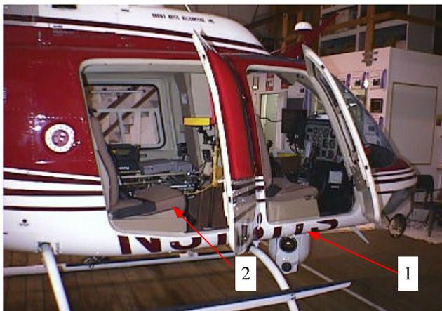
Figure 14. TIR Data collection system mounted on a Bell JetRanger Helicopter. A gyro-stabilized mount containing the FLIR and the visible band color video camera is attached to the underside of the helicopter (location 1). A computer, GPS, and digital video recorder are mounted on an equipment rack in the back seat (location 2).
