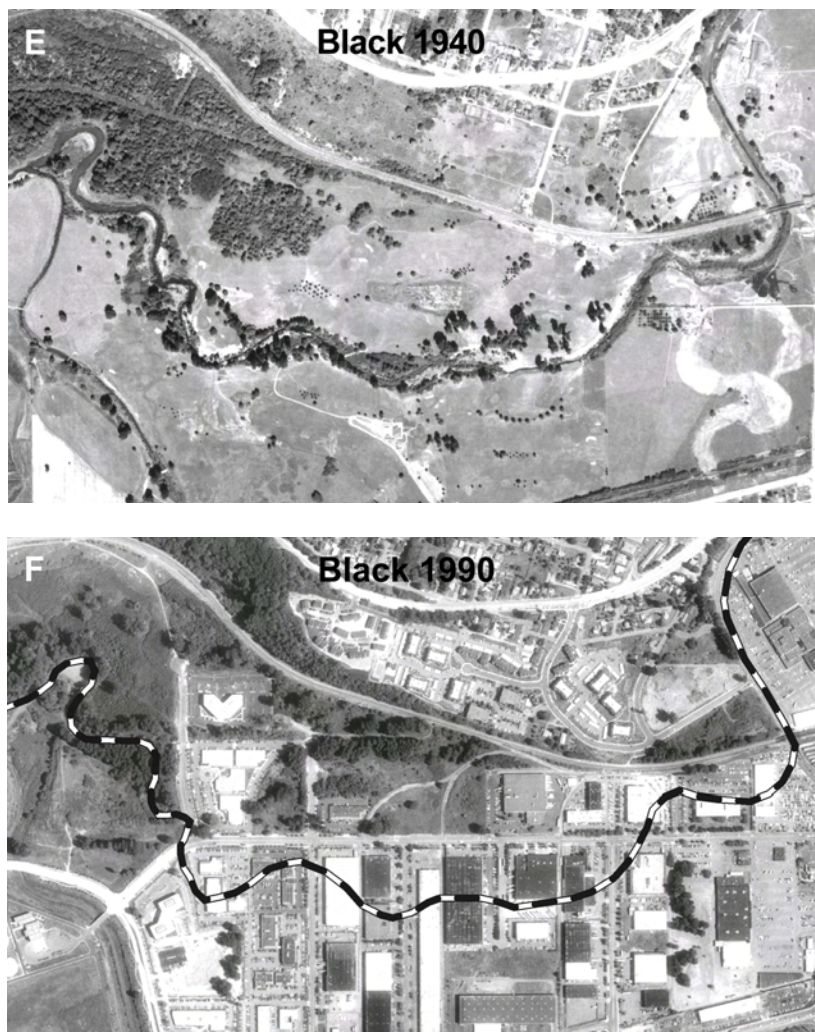
Figure 15 (continued). (E) The Black River retained a natural channel in 1940 with greatly reduced flow. (F) By 1990, the lower river retained a natural environment, but moving successively upstream, the former riverbed is covered by buildings, then becomes coincident with a street, and farthest upstream (out of view) buried by aviation runway.
