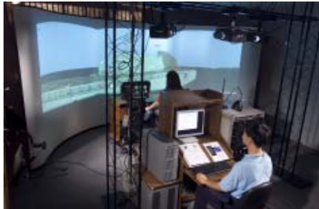
Figure 5. ART flight simulator with pilot in front of projection screen and operator at rear console
