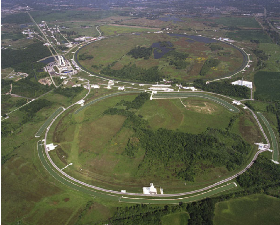
Photo 4: Aerial photograph of Fermi National Accelerator Laboratory (FNAL), at Batavia, Illinois. The beam originates at the top left and is accelerated in the linac (visible as a straight line) to get into the main injector (the bottom ring) where it is brought to 150 GeV. The Tevatron is the top ring, approximately 2 kilometers in diameter, where the beam is accelerated to 1 TeV. (Courtesy Fermi National Accelerator Laboratory.)
