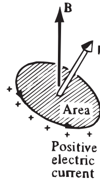
Figure 5.3: A current loop gives rise to a magnetic moment \mu . The direction of the magnetic moment is perpendicular to the plane bounded by the current.
