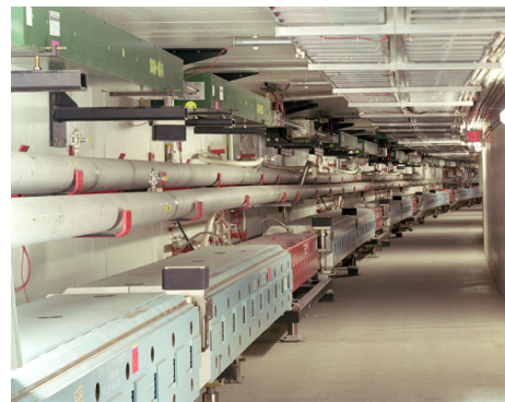
Photo 3: The photographs a-d show the essential parts of the 1 TeV proton synchrotron (Tevatron) at the Fermilab. Protons are accelerated to 750 keV in an electrostatic accelerator (Cockcroft–Walton, photo a); a linear accelerator (photo b) then brings the energy up to 400 MeV and injects the protons into a booster synchrotron. The booster synchrotron (photo c) raises the energy to about 8 GeV and the main ring (lower on photo d) to 150 GeV. The final energy of approximately 1 TeV is achieved in the Tevatron ring. [Courtesy Fermilab.]
