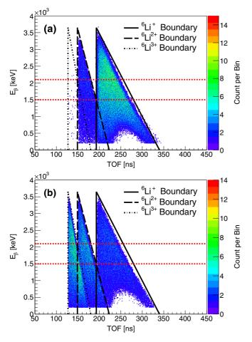
FIG. 2.  $E_{\beta}$  vs TOF 2D histograms for (a) data from measurements and (b) a Monte Carlo simulation assuming equal charge-state fractions. The boundaries for the three charge states are drawn in black lines, and the minimal  $E_{\beta}$  thresholds needed to separate the charge states are drawn in red lines. The lack of events near TOF = 250 ns and  $E_{\beta} < 750$  keV is due to the fiducial cut on the MCP.
