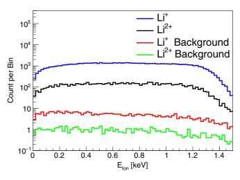
FIG. 4. <sup>6</sup>Li recoil ion initial energy distributions for Li<sup>+</sup> and Li<sup>2+</sup>. Background spectra are also plotted.
